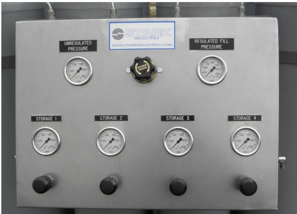
When more than four storage cylinders are used the best arrangement is to bundle them together in four groups of two, three or four to retain the usage of only four control valves and gauges. This arrangement keeps the operation simple while still achieving the benefits of the cascade filling process.
